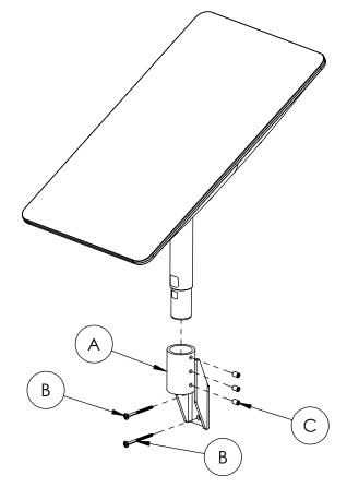
ATTACH THE SWM ARM TO A SUITABLE STRUCTURE WITH TWO RSS LAG SCREWS. MOUNT SHOULD BE LEVEL/PLUMB. SILICONE IS PROVIDED TO SEAL LAG SCREW PENETRATIONS FROM MOISTURE AS NEEDED.
