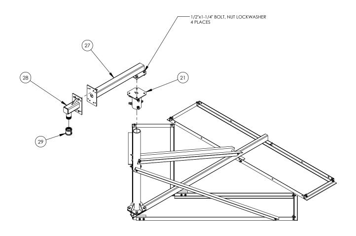
CLAMP THE CAMERA ARM ADAPTER SLEEVE TO THE MAST WITH SIX SET SCREWS. THE CAMERA ARM ASSEMBLY WILL SHIP AS AN ASSEMBLED SUB ASSEMBLY AND THE CONFIGURATION MAY VARY FROM THE DRAWINGSHOWN ABOVE BASED ON SPECIFIC PART NUMBER.
